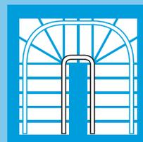
2000 Series. Fanned turns (90 or 180 degree spiral curve).
